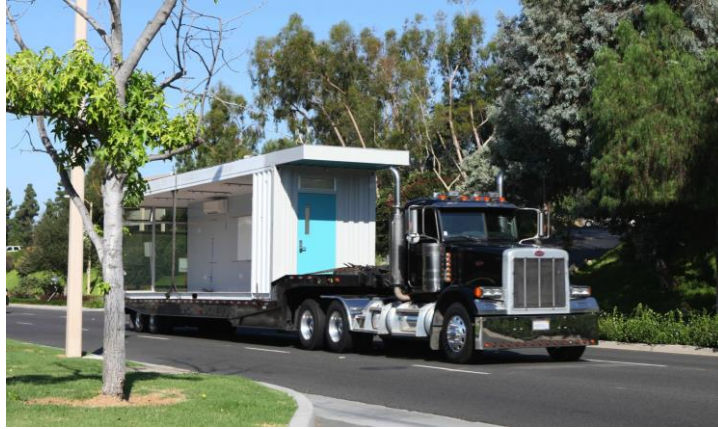
Figure 5. GrowthPoint prefabricated container arriving at construction site.
